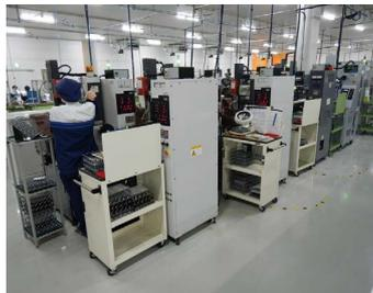
Electrical discharge machining line
